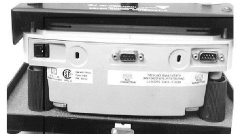
The rear panel of the UPM-DT Series provides power and RS-232 computer / printer connections. Adjustments to level the unit are made by rotating the rear stands.
