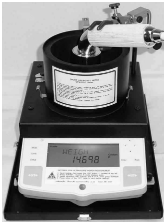
Front view of UPM-DT-1 & 10. Shown is the electronic balance, base assembly, test tank & transducer positioner.
