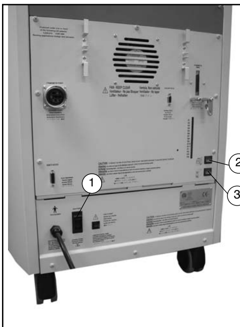
Figures 2.1 and 2.2: The main power(1), dynamometer power (2), computer power (3) and CPU (4) switches must all be turned ON to run the Advantage Software program.
