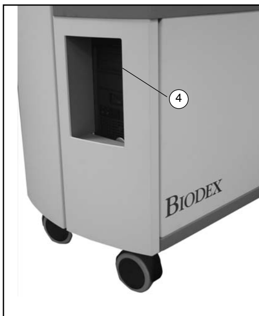
Figures 2.1 and 2.2: The main power(1), dynamometer power (2), computer power (3) and CPU (4) switches must all be turned ON to run the Advantage Software program.
