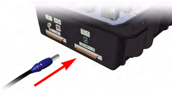
Figure 4. Connecting the Trigno Base Station power supply.
