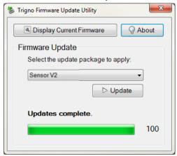
3. After updating the sensors and the base, launch EMGworks and pair the sensors. After a firmware update, all sensors must be re-paired to the base.
