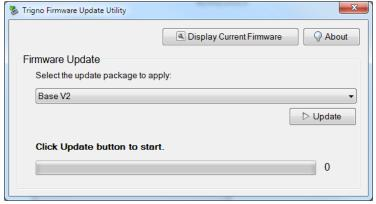
e. Each firmware component on the base will be updated. The base will reset several times during the upgrade process. Do not close the program, or disconnect the power or USB connection from the base while an update is taking place. The base update process takes approximately 2 minutes.
